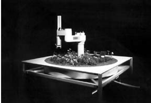
TeleGarden, industrial robot arm controlled via the Internet
