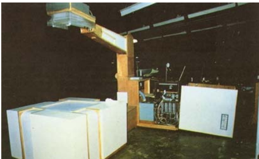
The cover of the electronics cabinet is open showing the computer and switching electronics. The column can erect to 17 feet and is about 14 feet across diagonally water collector base cabinet to the top of the electronics cabinet. It weighs about 1,500 pounds dry and was powered by 4,20 amp. 110 VAC, 60 cycle single phase electrical circuits.
