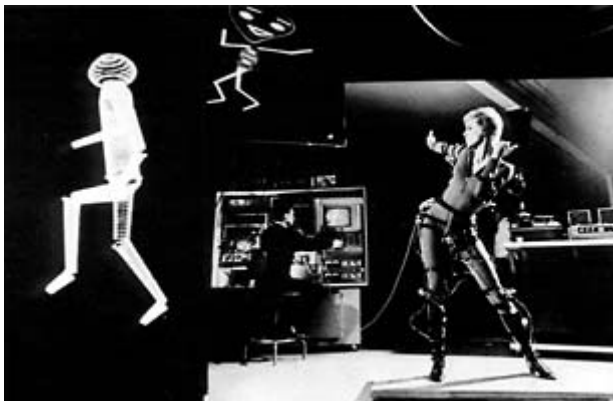
Lee Harrison III, photo montage featuring a dancer with body mounted sensors controlling real-time animation on the ANIMAC, 1962, Denver.
