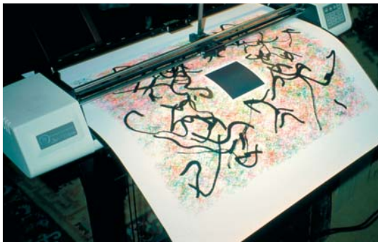
First coded brush strokes in 1987. Oriental brush mounted on drawing arm. Houston Instruments DMP 50 series pen plotter. Plotter driven with PC operating on DOS.
