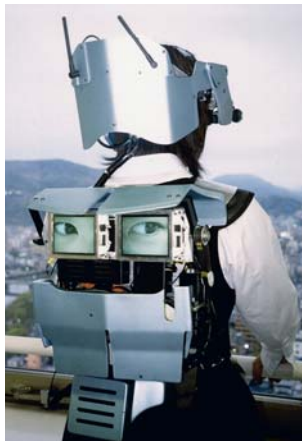
Dis-Armor, 2000: This instrument was used by high school students in Hiroshima. A microphone and two video cameras in the head piece transmit voice and images of the user's eyes to speakers and two LCD screens on his or her back. The piece also includes a rearview mirror, computer, and batteries, as well as wireless video transmission that allows pairs of users to wear each other's eyes and speak with each other's voices.
