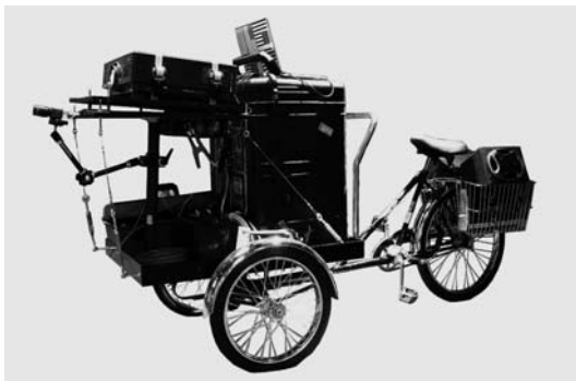
L.A.S.E.R. Tag (prototype) , March, 2007 Graffiti Research Lab, 2006 (James Powderly, Evan Roth, Theo Watson) 60 mw Green Laser, Digital Projector, Camera, Custom GNU Software
